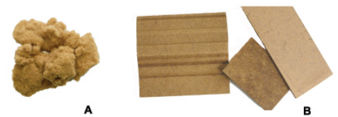
Fig. 4: A – Industrial fibre material B – Medium Density Fibre Board
